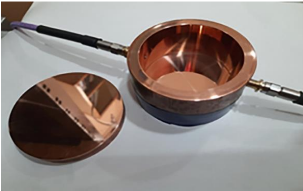
Fig. 1. An empty copper cylindrical resonator with a resonant frequency of 3.3 GHz with cover, coaxial input and output of high-frequency radiation.
