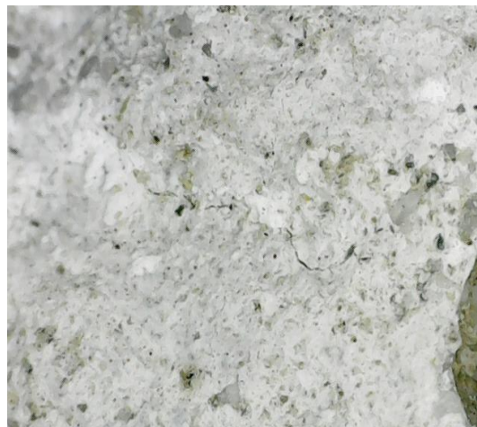
Figure 1. Structure of recycled aggregates at 500 times magnification. Microcracks on the surface of aggregate
