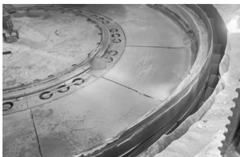
Figure 4. Wear pattern of the grinding table surface
