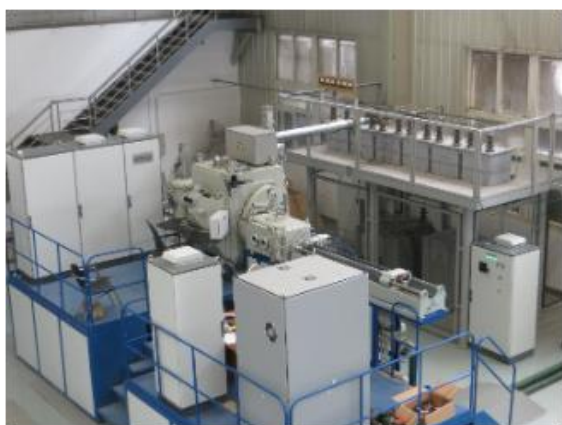
Fig. 2. Exterior view of the universal laboratory electron beam machine L-2.
