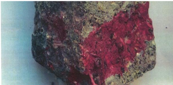
Fig. 3. Phenolphthalein indication of cement carbonation.
